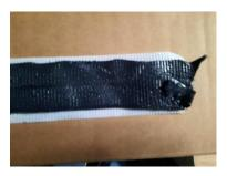
Mastic's do not set but stay flexible and pliable. This can result in the sealant "flowing" when it is under compression and then become visble as in the photo above.
